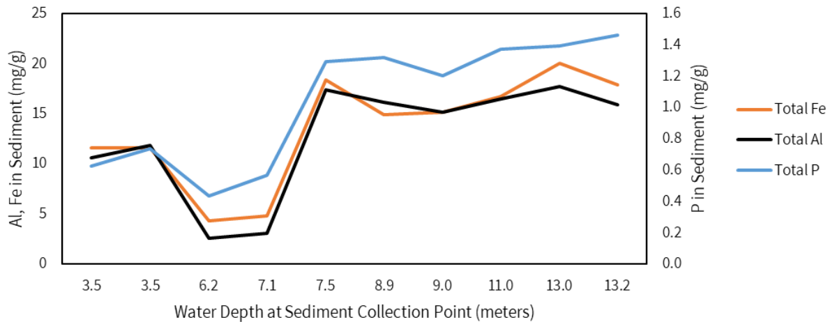
Figure 10. Total phosphorus, aluminum, and iron concentration (mg/g) in sediment cores (representing top 4 in or 10 cm) at various water depths across Lake Kanasatka. Refer to Table 4 for data and Figure 7 for locations.
