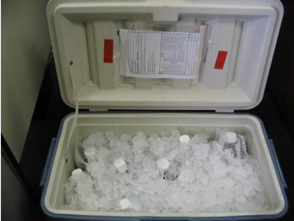
Figure 16. Stormwater samples packed for delivery to the lab, note the chain of custody forms attached to the lid.
