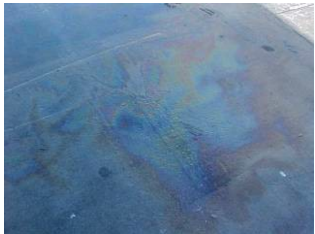
Figure 17. Example of oil sheen.
