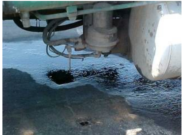
Figure 19. Example of vehicle leak.
