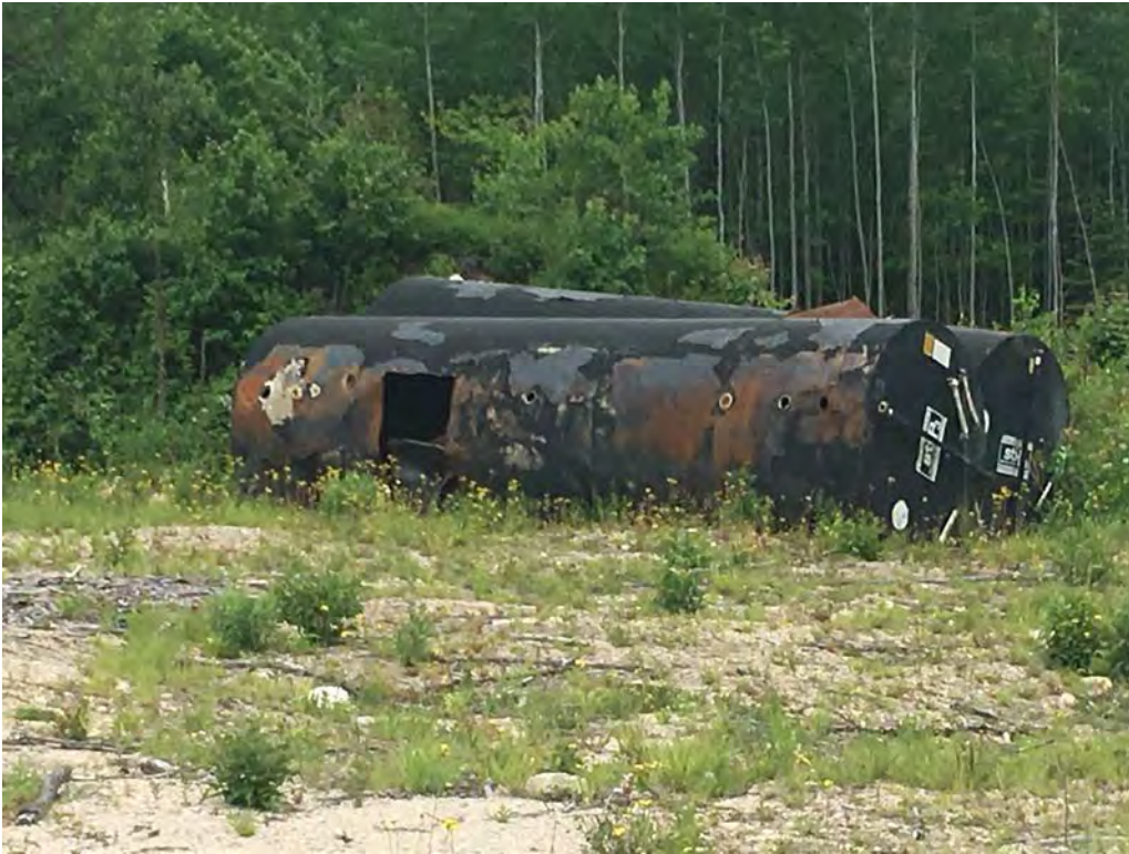
View of the two 10,000-gallon former underground storage tanks that were cut open and cleaned prior to transport from the former Littleton Sunoco facility.
