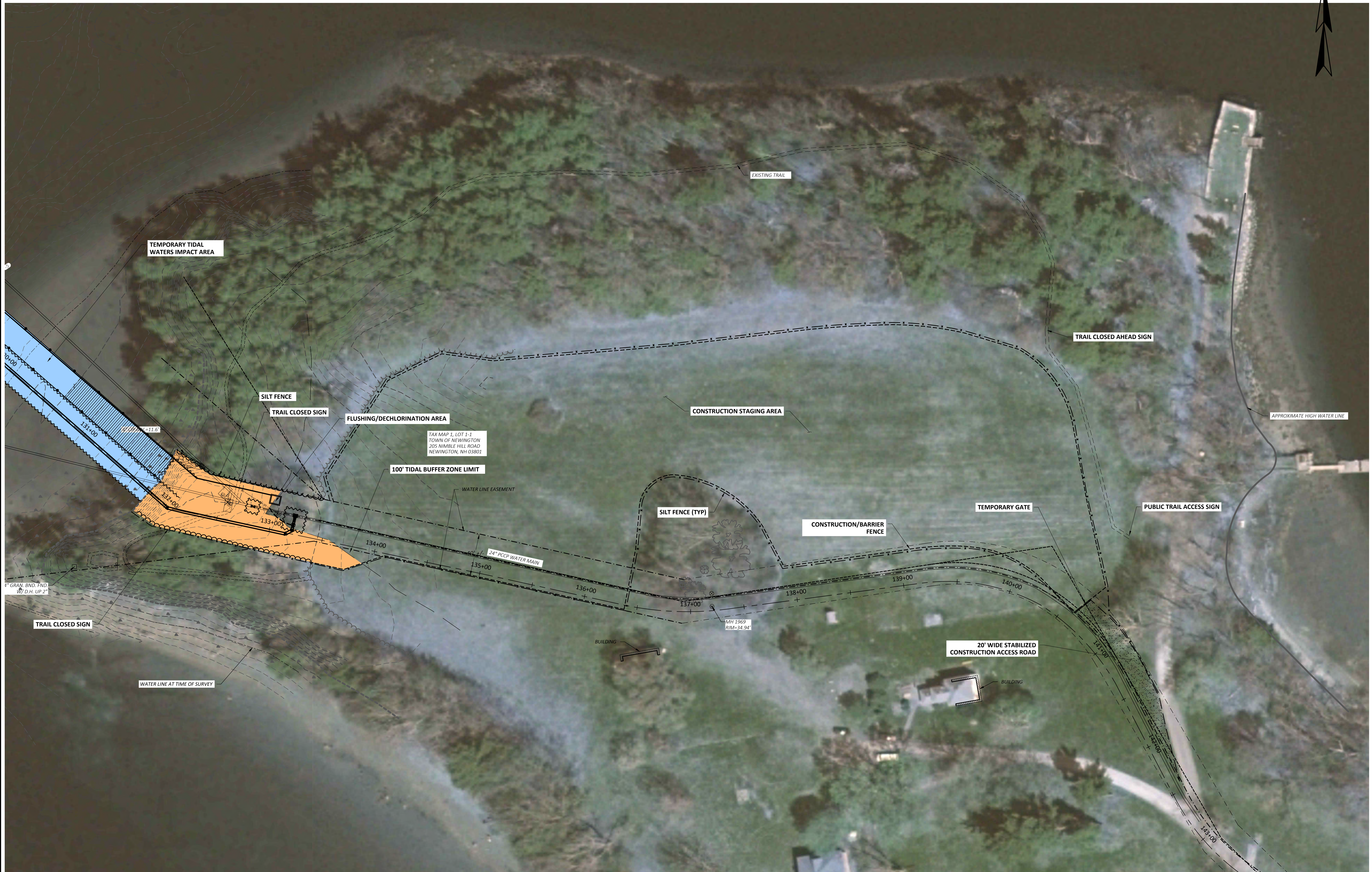
CONSTRUCTION STAGING PLAN-NEWINGTON SITE
