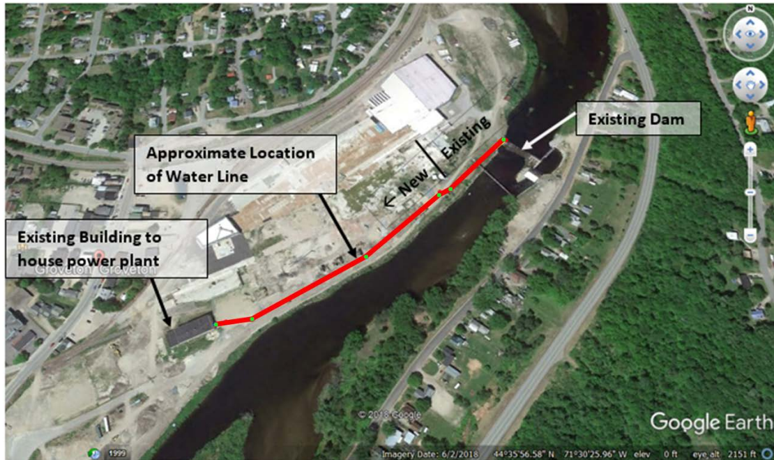
Figure 1: Google Earth aerial image showing the approximate location of the water line and existing building where hydrogen will be produced.
