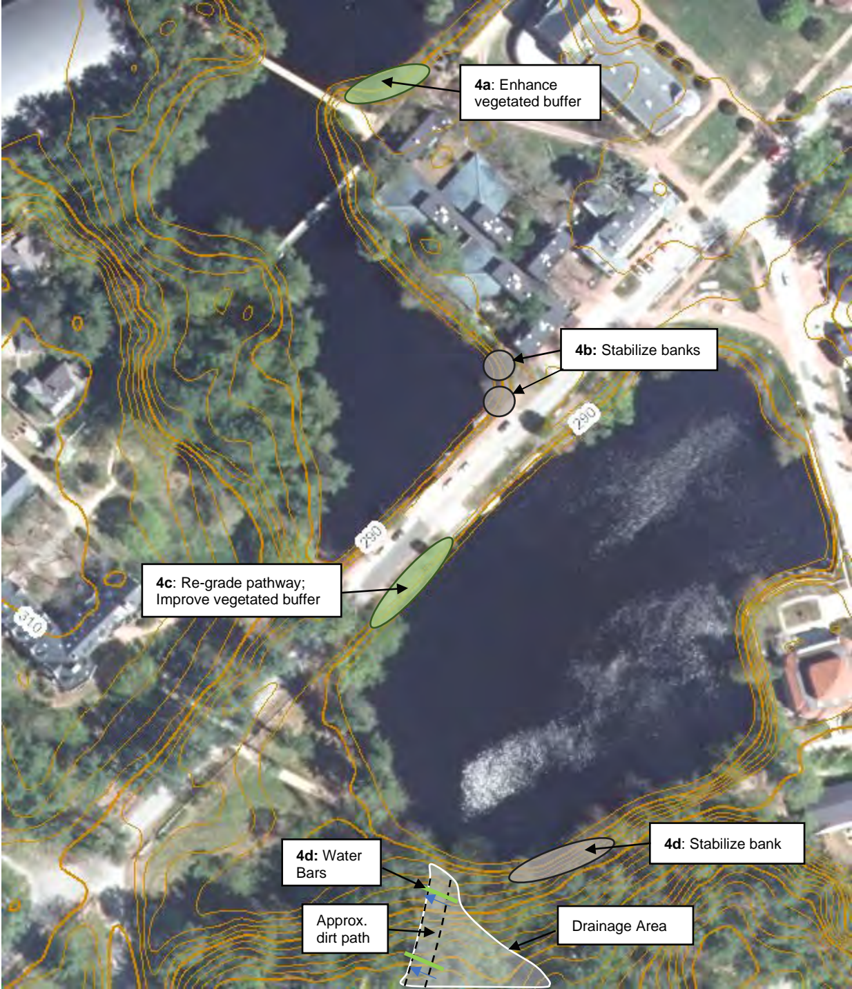
Photo 4-14: Proposed BMP configuration for sites 4a - 4d.
