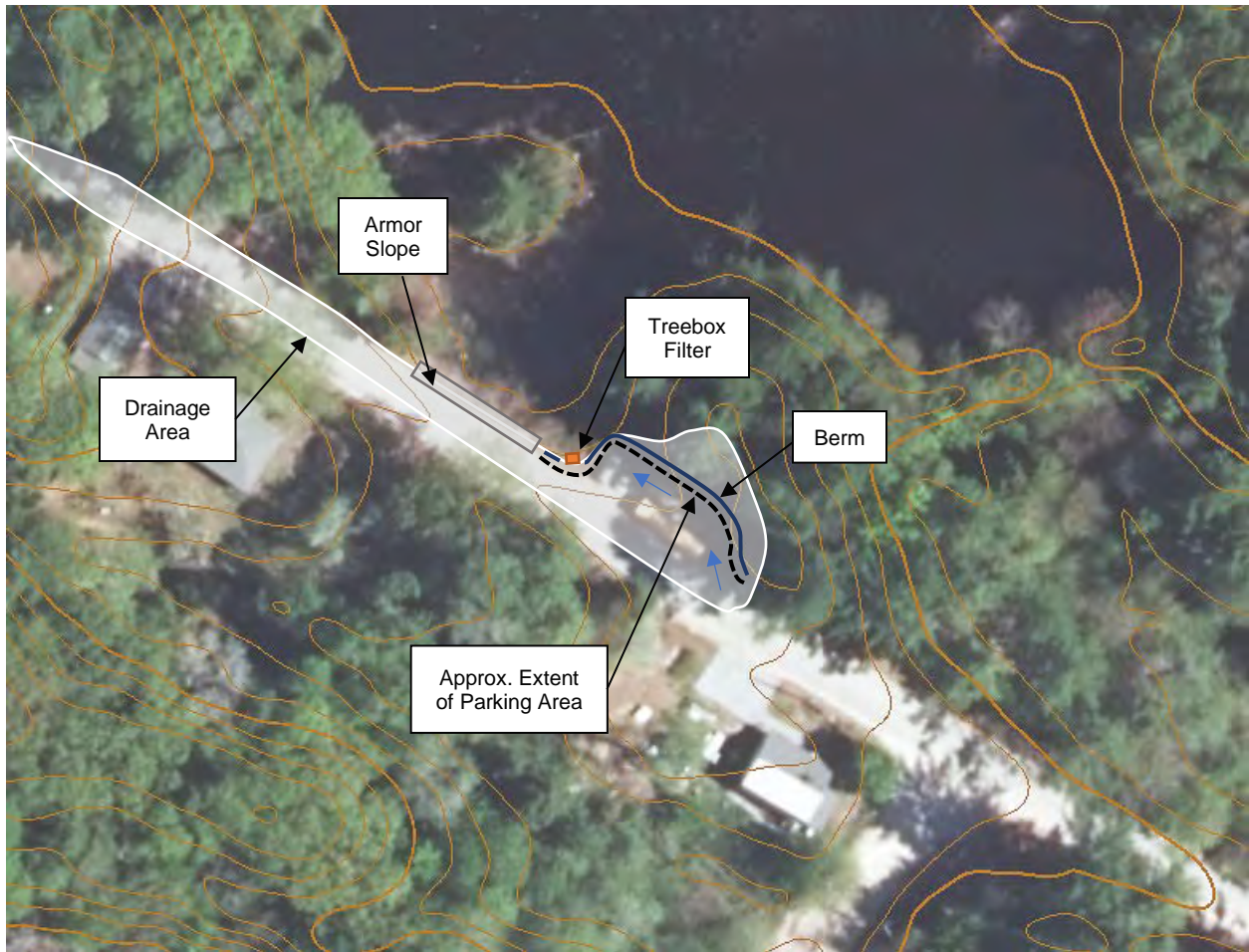
Photo 11-3: Proposed Area 11 BMP configuration.
