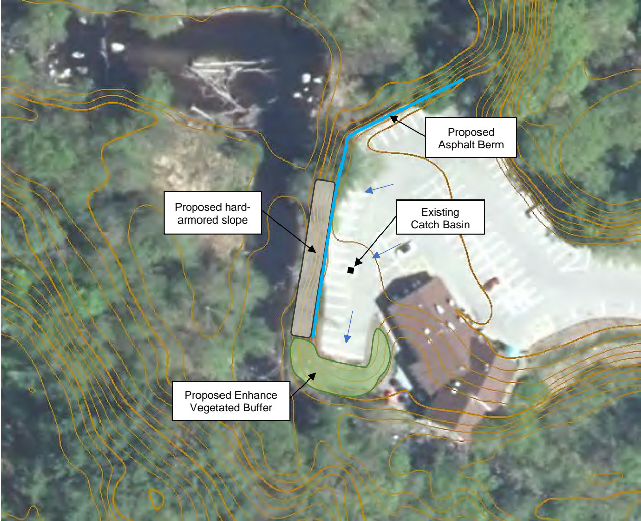
Photo 15-4: Proposed Area 15 BMP configuration.
