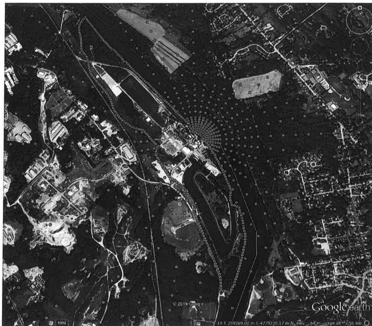
Figure 3 Modeling for 1-hour SO 2 SIP, Boundary Receptor Network and Inner Polar Grid
