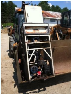
50' vintage dispenser, post removal.
