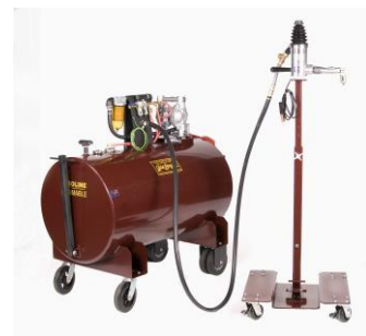
Picture of a gas buggy and drill system.
