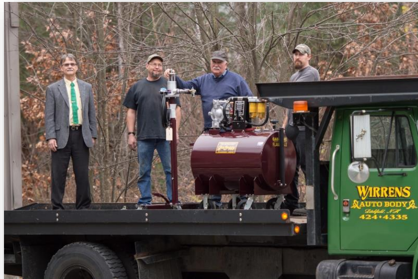
A gas buggy and fuel tank drill system being picked up by Warren's Auto Body. Note the dual fuel filter assembly improvement added to the NHDES order.
