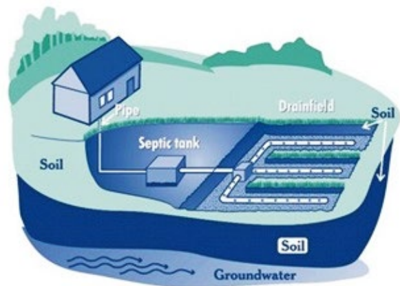
Figure 14. Conventional septic system and leachfield
