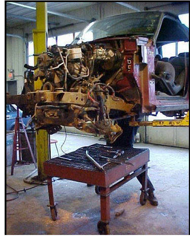
Dismantle vehicles over a concrete surface and use drain tables to fully drain parts
