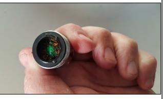
Picture of an aerator with particulate
