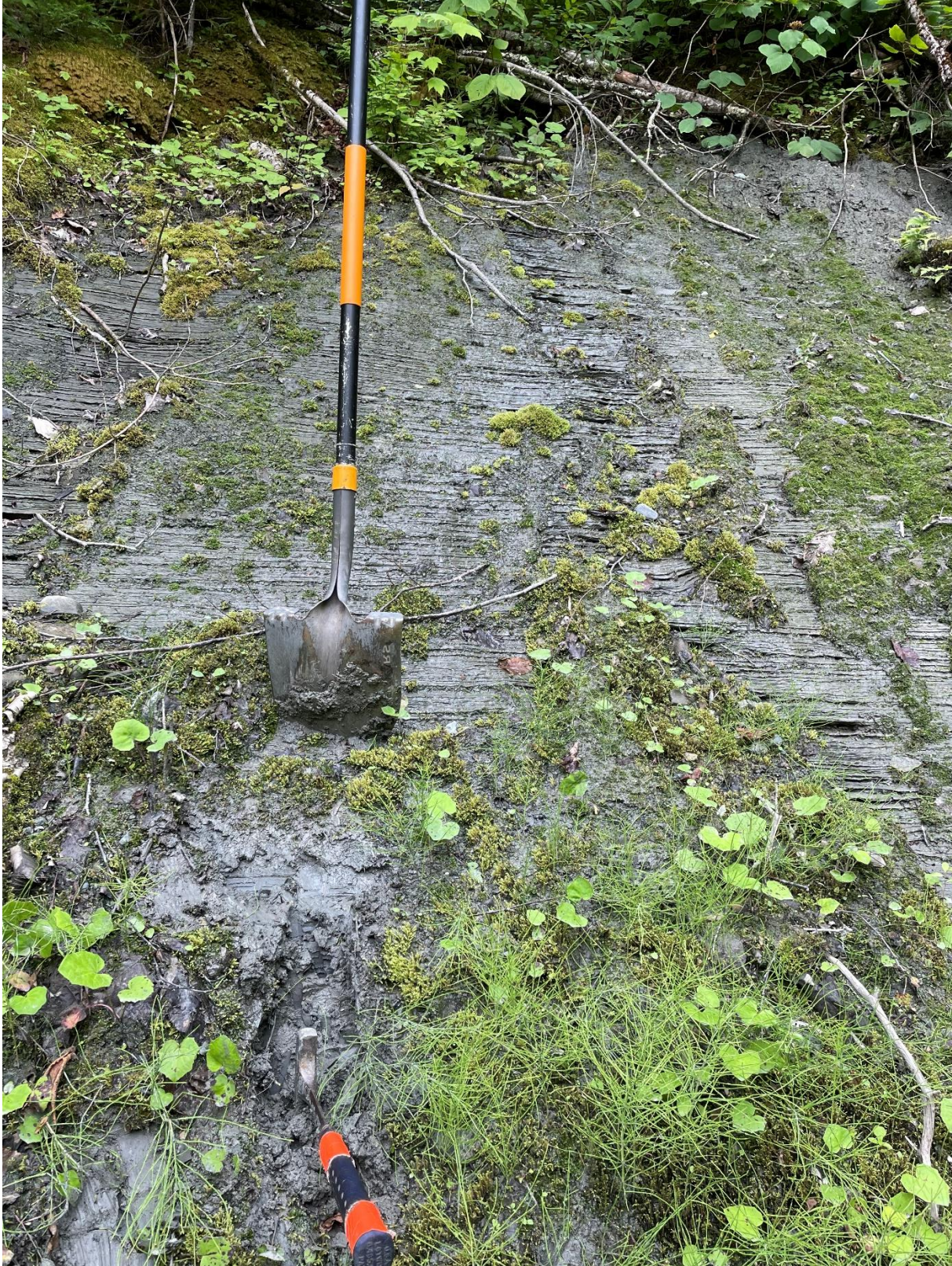
Figure 12. Photograph looking west at exposed section of laminated clays with silt and sand partings in Little Tunnel Brook ravine (2000-ft elevation, 44° 03.3314' N, 71° 50.1438' W).
