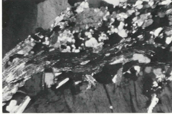
Figure 13. Zone of crushed minerals exhibiting mortar structure and secondary muscovite oriented parallel to plane of granulation. Sample no. 32, from two-mica granite, 3,500 feet north of intersection of Lane Road and route 102, Chester, N.H.
