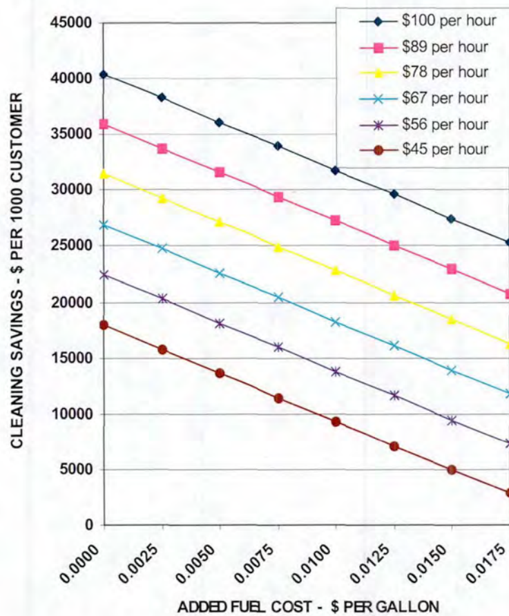
Figure 3-5: Net Cost savings per 1,000 Houses Using Low Sulfur Oil For: 0.25%S (initial) and 865 Gal per Year
