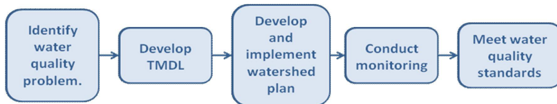
Figure 6-2: Relationship between TMDLs and Watershed Management Plans (USEPA, 2008).
