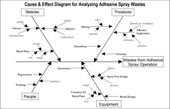
The planning team went back to the adhesive spray process to examine the potential causes they had identified. The team found that the conventional spray equipment, application techniques and mixing procedures appeared to have the most significant effect on waste generation. With these major cause categories in mind, it was time for the team to do some **BRAINSTORMING** to come up with possible alternatives to the current process.
