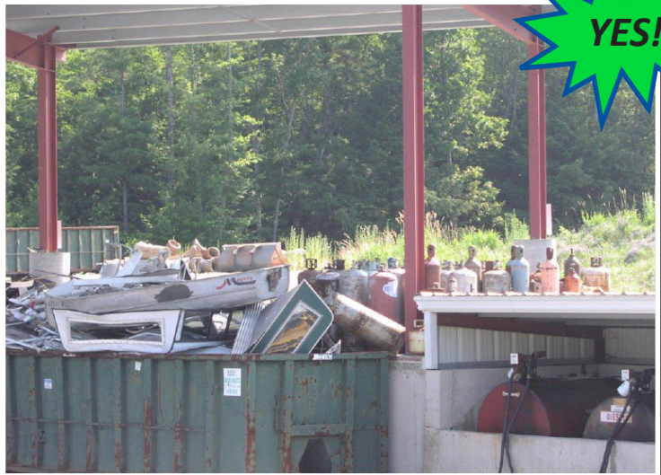
By collecting scrap metal in a transportation container, you keep it off the ground and only have to handle it once before sending it to a scrap metal dealer. The container is under a roof to keep out precipitation.
