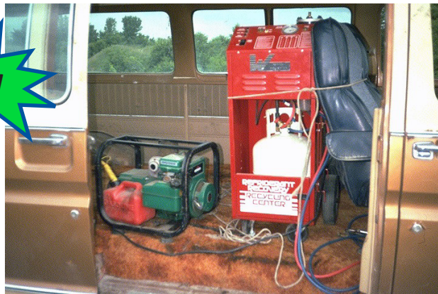
You can hire mobile contractors to remove refrigerants. The contractors travel from site to site performing this service. Make sure they are certified and have approved equipment.
