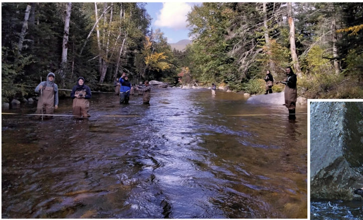
ABOVE: PSU students measure streamflow at three transects below the NHDES streamflow station on the upper Ammonoosuc River in Crawford's Purchase. (Photo by Joe Schmidl) RIGHT: PSU student Gavin McNabb (left) and NHDES fluvial hydrologist Joe Schmidl measure the depth of the sensor. (Photo by Lisa Doner)
