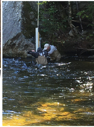
ABOVE: PSU students measure streamflow at three transects below the NHDES streamflow station on the upper Ammonoosuc River in Crawford's Purchase. (Photo by Joe Schmidl) RIGHT: PSU student Gavin McNabb (left) and NHDES fluvial hydrologist Joe Schmidl measure the depth of the sensor. (Photo by Lisa Doner)
