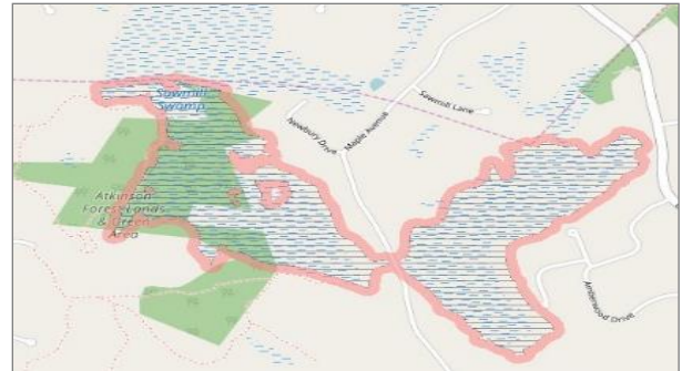
Figure 5. The duly-established 100-ft buffer for certain designated prime wetlands is shown as a pink band in the WPPT.
