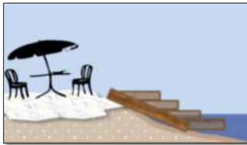
Figure 5 - Access stairs to and from water access structures, viewed as a cross-section. Steps made from stone, concrete or similar materials leading to the water may be incorporated in the design of a water access structures, but must not exceed six feet in width.
