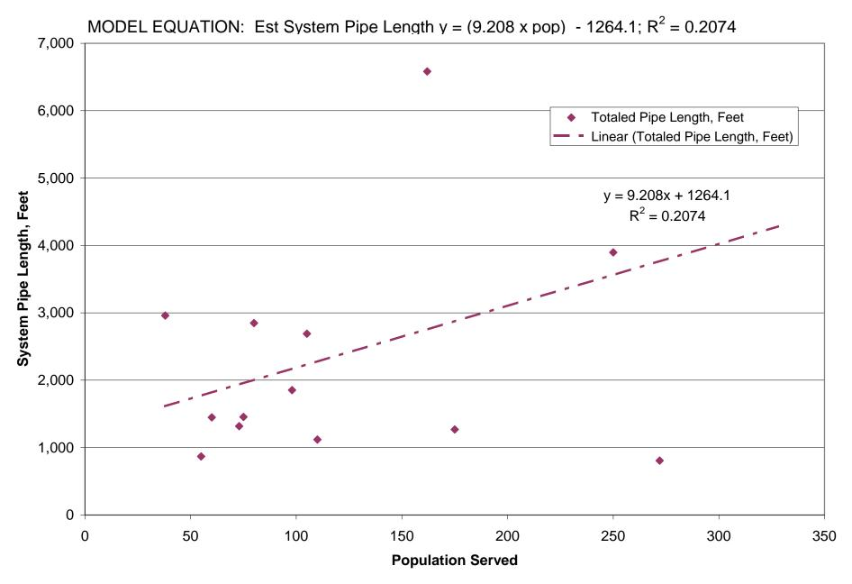
Figure A-3: NH Systems w/ No Fire Protection
