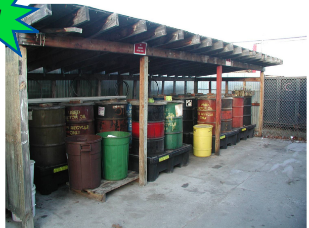
Drums are correctly labeled, have secondary containment and are on a concrete surface, covered by a roof.
