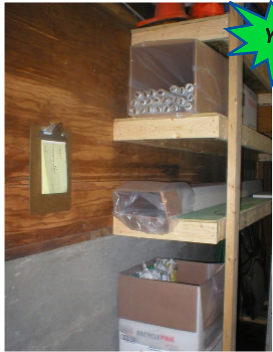
Place fluorescent lamps/bulbs inside a structure that shelters them from the weather, stored inside sturdy containers and closed except when lamps are being added. (Boxes are open to show lamps inside.)
