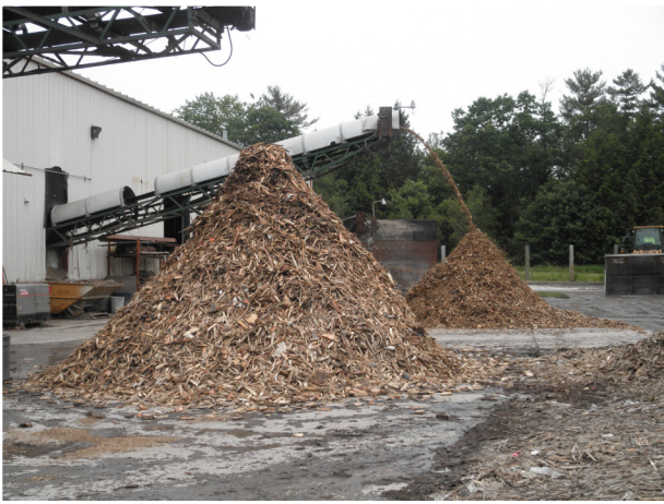
This C&D wood waste has been processed into a recyclable material, for use in manufactured wood products such as chip board.
