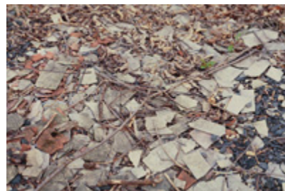
Asbestos sheet scrap dumped on ground surface
