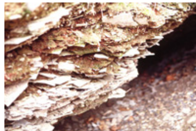
Moss covered asbestos sheet scrap protruding from embankment
