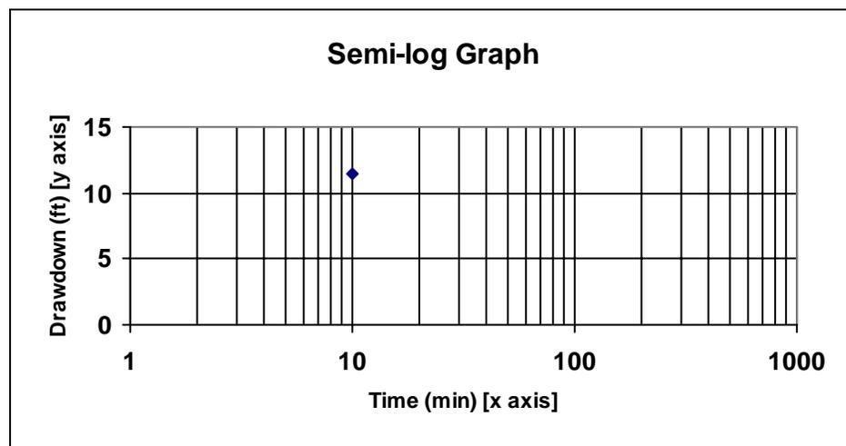
The rest of the measurements are then plotted the same way. Sample Plot 1 employs the data points listed in the table below. For simplicity, only four drawdown measurements are plotted. Use all the measurements taken during the pumping test.
