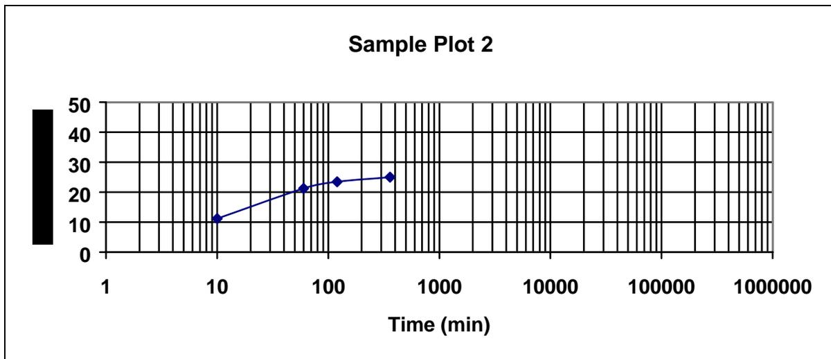
Draw a best-fit line by laying a ruler along the data points taken from the last 12 to 36 hours of the test and marking a straight line through them. Extend the straight line out to the 180-day point, or 259,200 minutes, as shown in Sample Plot 3.
