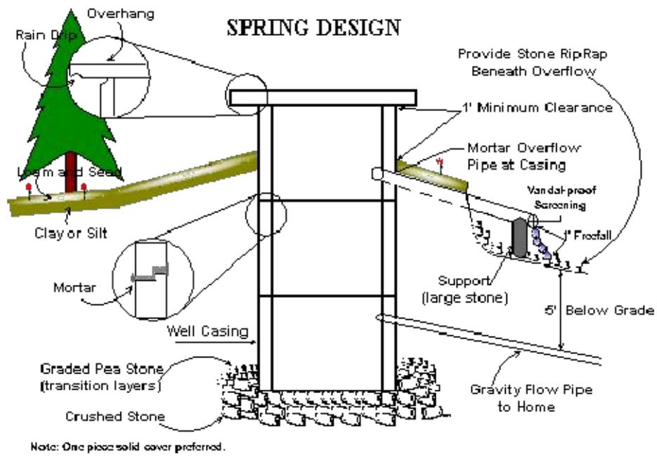
**Figure 1. Spring Well Design Components.**
