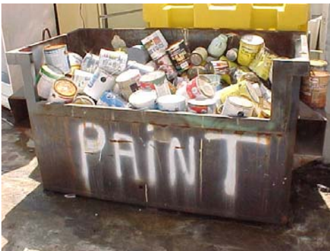
Cans may be disposed of as a solid waste or recycled, if completely emptied of any free liquids.
