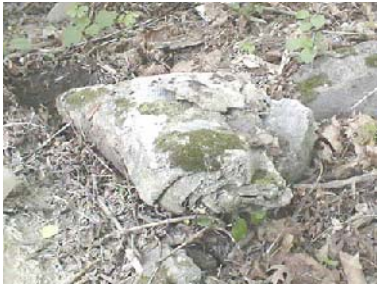
A partially buried rolled sheet of asbestos.
